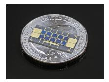
TriLumina 300W output VCSEL Module (8mm x 16mm)
