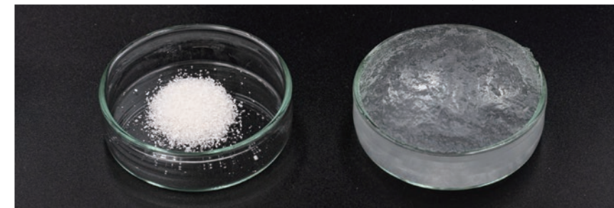
NAGASE-developed SAP, which is made using a high percentage of bio-derived raw material, before and after absorbing water (left and right, respectively)
