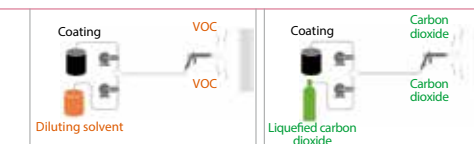
Figure 1 Solvent Coating (Traditional)
