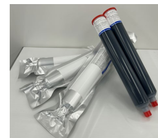
LMC: Liquid Molding Compound
