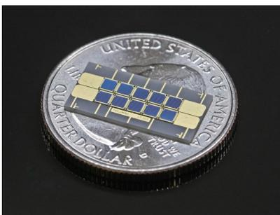
TriLumina 300W output VCSEL Module (8mm x 16mm)
