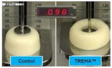
Hardness of rice cakes are compared at the equivalent pressure by using a rheometer.
