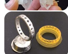
3D Printed Molding Examples Using UV-Curable 3D Resins
