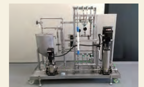
Solvent-resistant separation membrane process test equipment
