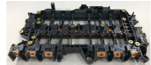
Metal insert mold parts for automotive inverters
